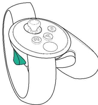
Figure 32 - The controller trigger allows you to interact with the menus and tools
